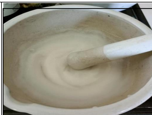
Fig. 6: Mixing the oil phase and water phase
